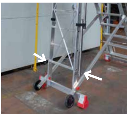
Bokada stabilizatora. Closed stabilisers.
